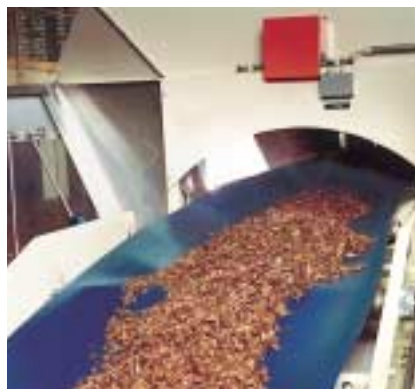
Horizontal conveying with troughable belts. The tension member construction provides the flexibility in the desired direction.
