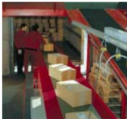
Left: Belts for telescopic conveyors – here being used to unload lorries – must be designed to run with counter bending and at the same time, to withstand high punctual loads.
