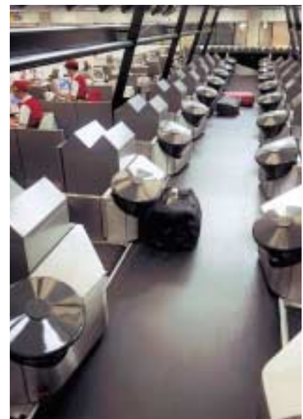
Below: Collecting belt in check-in area of an airport. The good flatness of the belt type here ensures that the goods can be discharged to the side smoothly, even on wide belts. Flame retardance is a “must” in modern airports.
